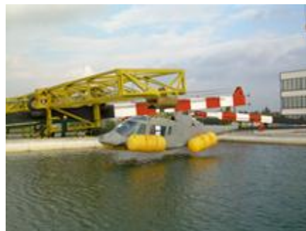
Figure 3: Full scale helicopter crash and ditching test
