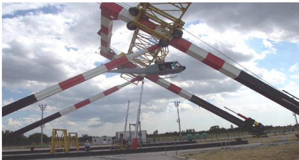
Figure 3: Full scale helicopter crash and ditching test
