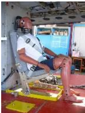
Fig. 4 LISA instrumentation (anthropomorphic test dummies, high speed cameras, data acquisition system)
