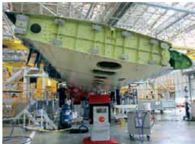
The TAM Group designed and manufactured tools and performed machining, beveling, drilling and laser tracker inspection of fairings and flap actuators. It continuously performed 5-axel machining of these carbon fiber fairings, whose principle purpose in the aircraft is to shelter and partially support the mechanism for flaps extention and retraction.
