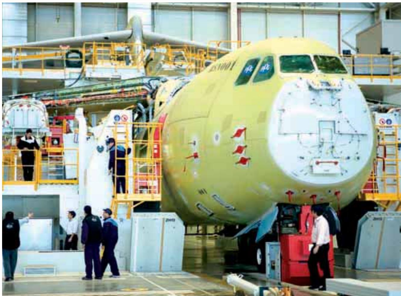
In the area of entire aircraft structural tests to be carried out at EADS CASA facilities in Getafe, the testing specimen and the testing bed were completely assembled, including actuators and measuring equipment, with testing scheduled to start at the beginning of 2008.
