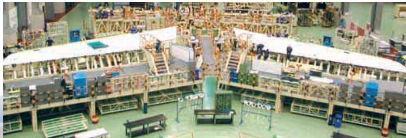
SISTEPLANT collaborated with AIRBUS ESPAÑA at its facilities in Illescas in redefining productive flows, with the objective of reducing movements and simplifying handling operations of large volumes of parts and tools.
