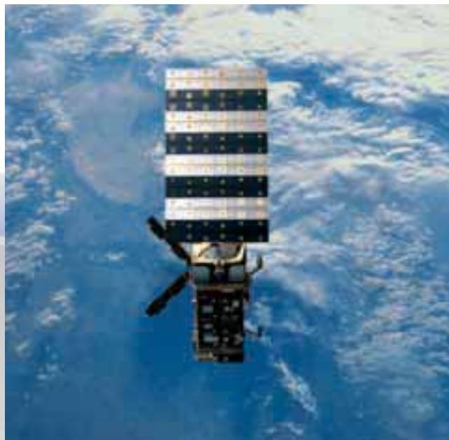
SENER, within the complete attitude and orbit control system (ACMS/AOCS), for Thales Alenia Space France as the final integrator and Thales Alenia Space Italy and ESA as clients, entirely developed the system that automatically determines and controls the position, stability and targeting of the Herschel and Planck satellites.
