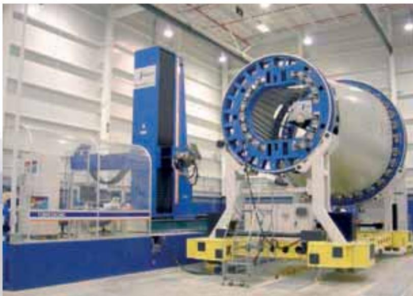
In 2007, TECNATOM kept its commitment to technological development with the purpose of assuring highest support to the manufacture of carbon-fiber aeronautical components, delivering equipment and inspection technology with non-destructive testing, especially ultrasound.
